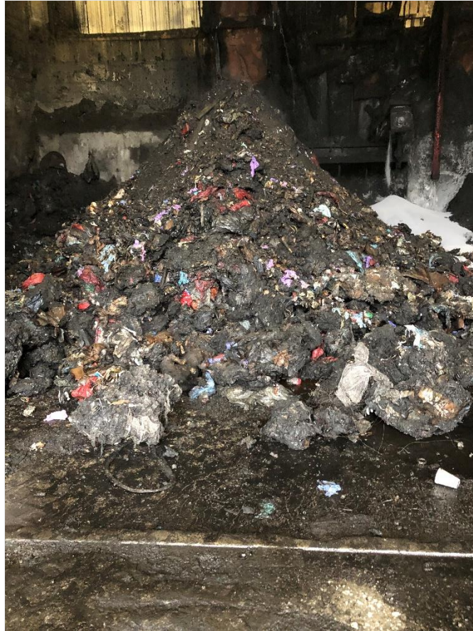
Insufficiently incinerated special medical waste on ash pad floor, September 27, 2019
